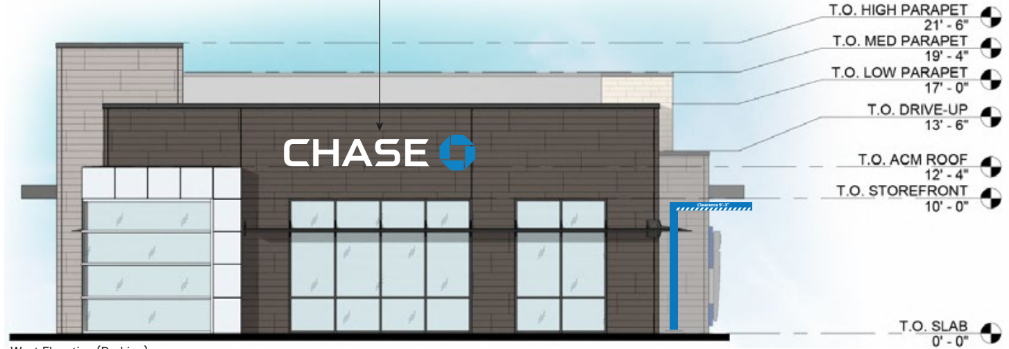
West Elevation (Parking)
